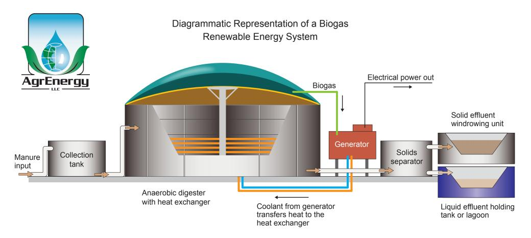
Collection tank: Manure and other organic farm waste is collected in a tank. If necessary water is added to the waste so it is easy to pump through the system.
