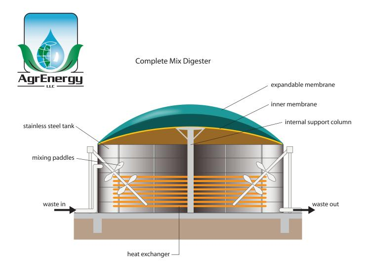
A complete mix organic digester is a continuous mix biogas production system. Manure moves through the system in a continuous flow. As new waste enters the tank, old waste is removed. Biogas production proceeds without any interruption from the loading of the farm waste and unloading of the effluent material.
